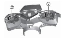
5. Push in on the burned-out bulb, turn it counterclockwise, and pull it out.
