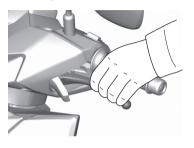
Pull the brake lock lever from below with your right hand (1) and release the combined brake lever. (2) (Hold the brake lock lever in the same position with your right hand.)
