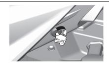
Insert the fuel nozzle ① into the refueling port until it reaches the bottom ② (where the fuel nozzle stops), and refuel.
