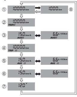
Press the **SEL switch** or **MODE switch** to set each item in the combination system display.
