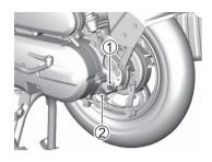
NOTE: If oil is dirty with sludge or used for a long period, drain the oil by removing the drain plug ② and pour fresh oil through the oil level hole.
