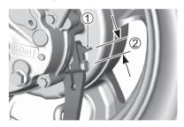
If the indicator is beyond the range, the brake shoe assembly should be replaced by your Suzuki dealer to ensure safe operation.
