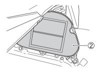
Inspect the air cleaner element condition. Replace the air cleaner element periodically.
