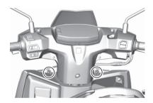
4. Unhook the hooks and remove the front leg shield ①.
