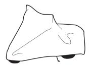
NOTE: Apply the body cover after the engine and muffler have cooled.
